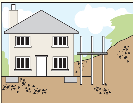
Fig. 4 Scaffold poles grouted into grid of steel tubular piles of working platform constructed.
