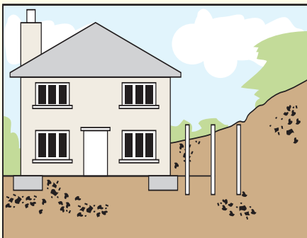
Fig. 3 100mm dia. steel tubular piles.
